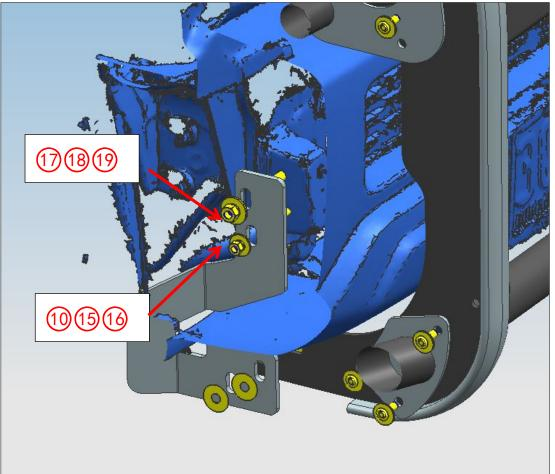
Step 2: Install Support Brackets 89 on the car with standard parts 1621221521 according to the following figure. (L & R symmetry)
