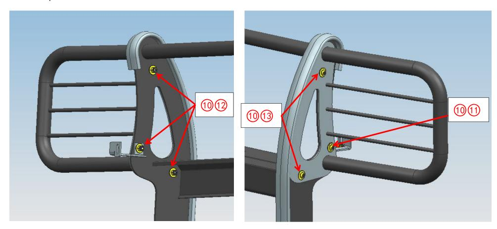
Step 4: Install the Lower Brush Guard 45 to the Front Guard 1 with standard parts 10131012. Do not fully tighten the hardware at this step.
