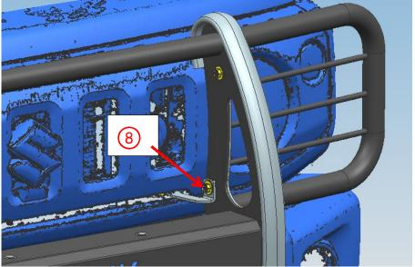
Step 3: Install the Upper Brush Guards 23 to the Front Guard 1 with standard parts 1011302. Do not fully tighten the standard parts at this step.
