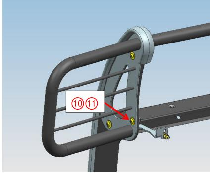
Step 6: Adjust the guard and fully tighten all the standard parts. Complete Installation.
